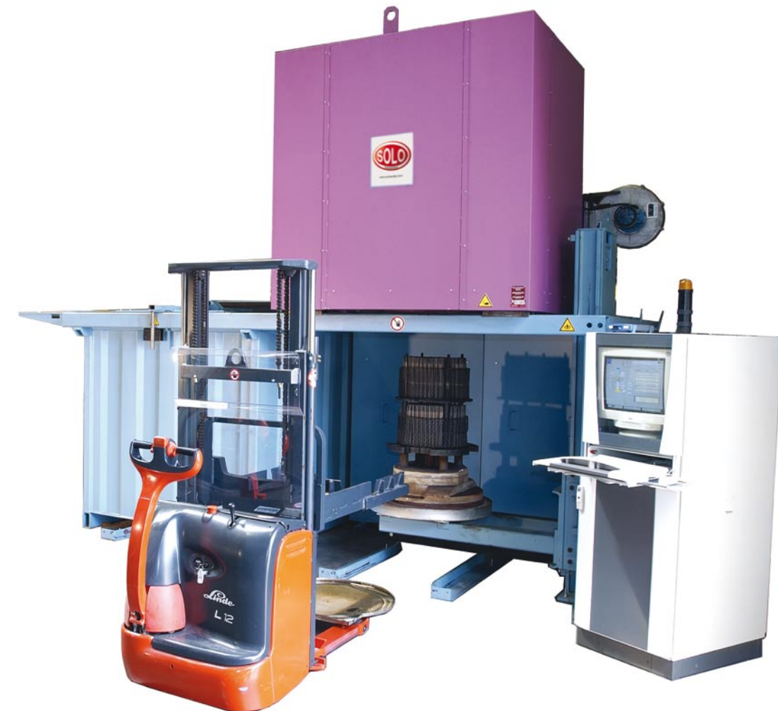
SOLO® Bell-type furnace manufactured under license by Thermic Service SA
