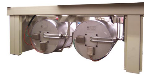
2 integrated NH 3 crackers
